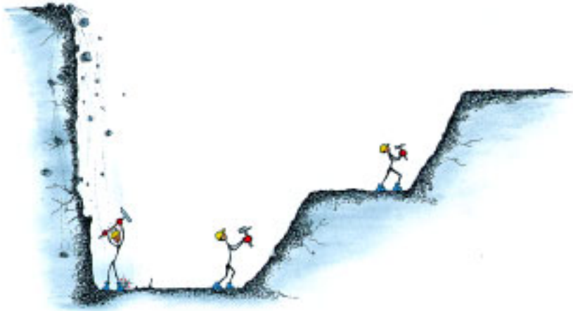
Unsafe steep pit wall.
