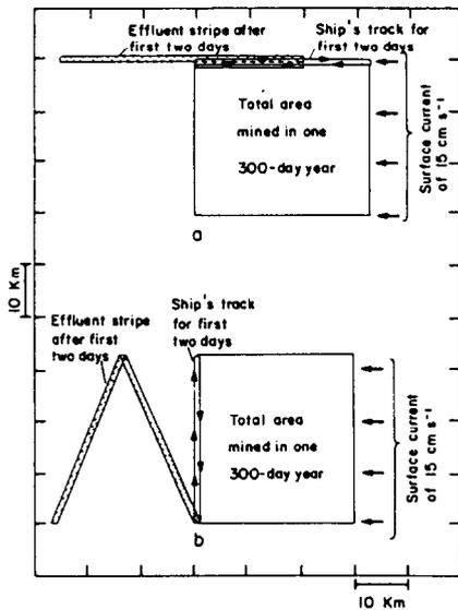
Figure 5. Configuration of effluent stripe after two days of mining with surface current (a) parallel to the ship's track, and (b) normal to ship's track.
